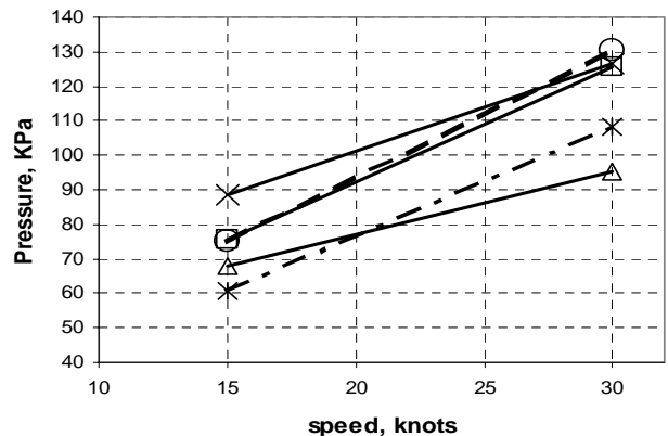
Figure 14: Maximum pressure, keel fwd, 15 and 30 kn, light displacement, 11 ft (3.35m) waves
