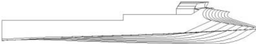
Figure 2: Profile and Buttock Lines of the Wave Piercing Hull - Bow B (Short)
