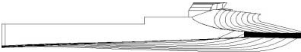
Figure 3: Profile and Buttock Lines of the Wave Piercing Hull - Bow C ("Duck Bill")
