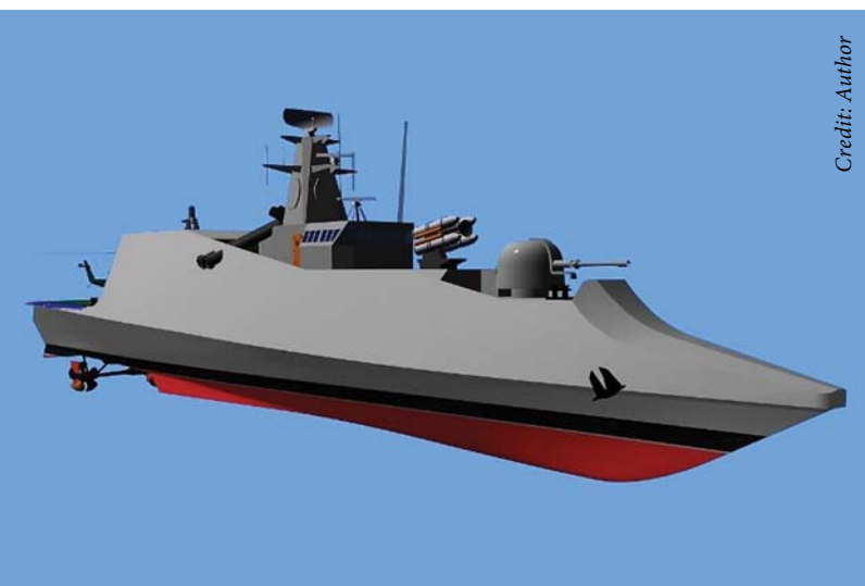
Design of a future Fast Attack Corvette with advanced wave-piercing hull form.
